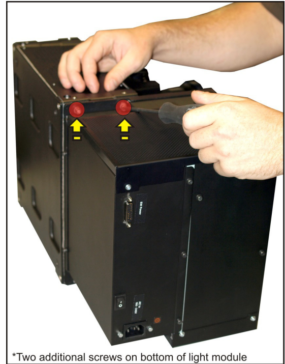
*Two additional screws on bottom of light module
